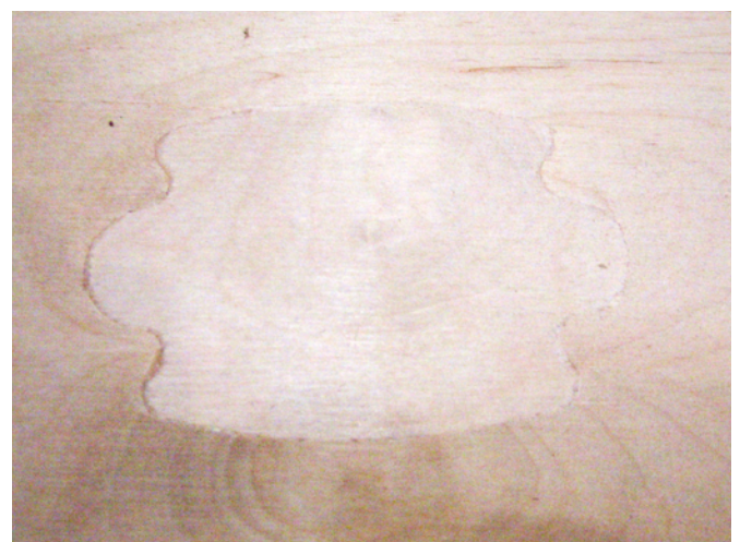
A 'Batman' shaped plug or patch – often found on BB Grade Plywood and lower. These patches are generally well made and give a sound/solid face.
